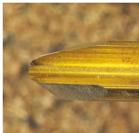
▲ Pic.18 You can just see the top wing on the gouge has been dulled off. As soon as you can see a cutting edge 'looking back at you' it's time for a sharpen
